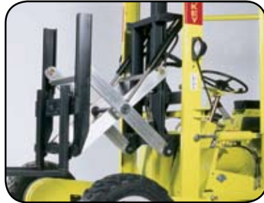
Intelligent use of aluminum on scissor units keeps weight low and strength high. Pallet, lumber, brick or other specialty forks available.
