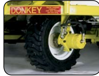
The optional on-demand third wheel drive increases gradeability, traction, and sharp turn capability. (Standard on M13-5K)
