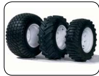
Flotation tires (left) for delicate terrain, terra tread (middle) for improved traction, standard (right) for normal use.
